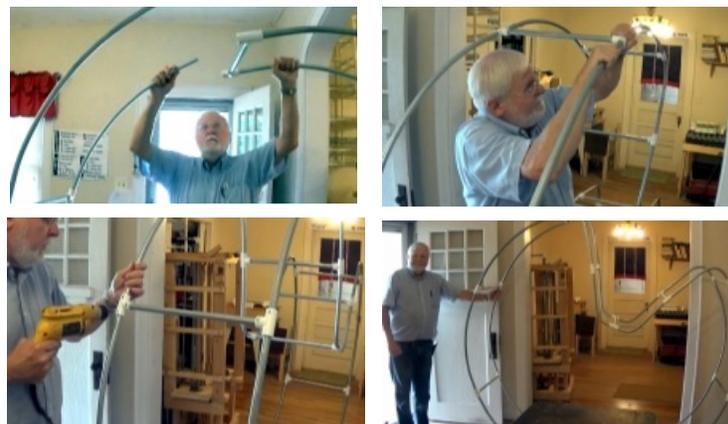
After the final two big bends are inserted and before screws are added, bring the opposite side of the unit up and around to connect with the last two big bends. You might have to push down on the top of the unit to allow the big bends to easily fit into the tee post openings on the other side of the unit. Put them in place, then insert the remaining four screws to complete the unit.
