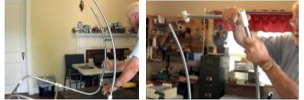
opposite direction and insert screws adjacent to the curved parts of the medium bends. The first screws on the newly added tee post can then be inserted. Do the same thing to the other side. Be sure that all screws will be on the outside of the frame unit.
