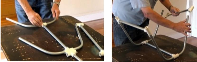
2. Start with the wedge portion of the frame, inserting the curved edges of the small bends into both ends of a tee post. Raise the remaining ends of the small bends and attach a tee post to the left and right sides, to separate the upper and lower rail, forming a "U" shape. The pre-drilled holes in the tees should be visible from the inside of the "U."
