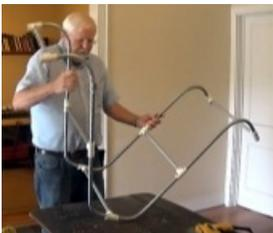
5. You are now working with four connect points, the upper and lower rail on both the right- and left-handed sides. On one side, take two big bends and insert them into the edge tee post, the big bends facing up. Put another tee post on the open ends to keep alignment, then flip the unit into the first
