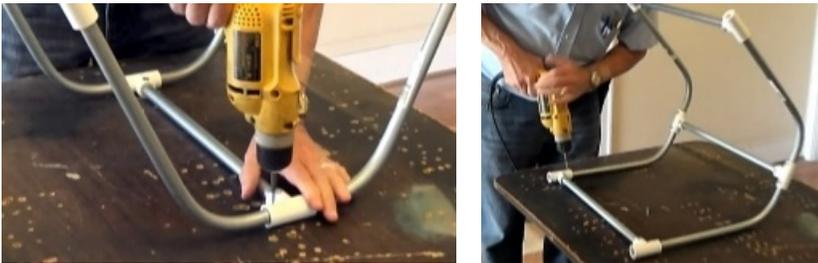
3. Now, using the power driver, drill screws into the bottom tee post and then rotate the two sides onto a flat surface to drill one screw on each side tee post where it connects with the small bend. Always be sure the rails (curved metal) are inserted all the way.
